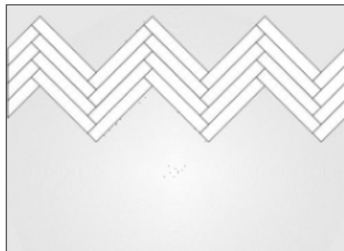
Figure 9: Complete four rows. Install additional rows to complete four full rows.
