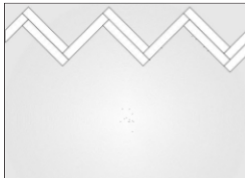
Figure 7: Install the A-panels. Continue from the left to the right and install all the A-panels in the second row. Finish with a piece of panel cut to size (step 5).
