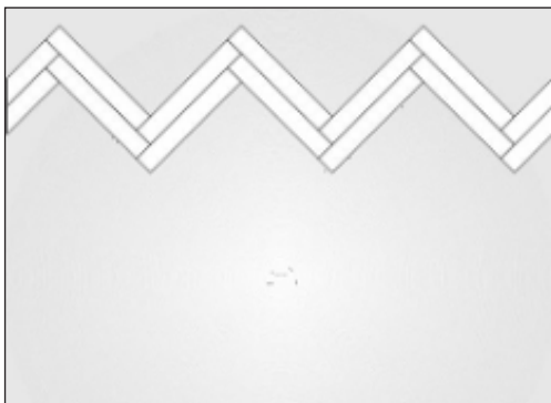
Figure 8: Continue with the B-panels. Now work in the opposite direction, from the right to the left and install all the B-panels in the second row. Finish with a piece of panel cut to size (step 5).
