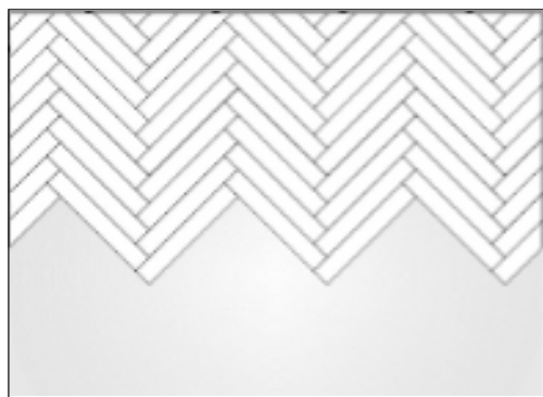
Figure 15: Subsequent rows. Start each subsequent row by installing the A-panels from the left to the right and complete the row by laying the B-panels from the right to the left.
